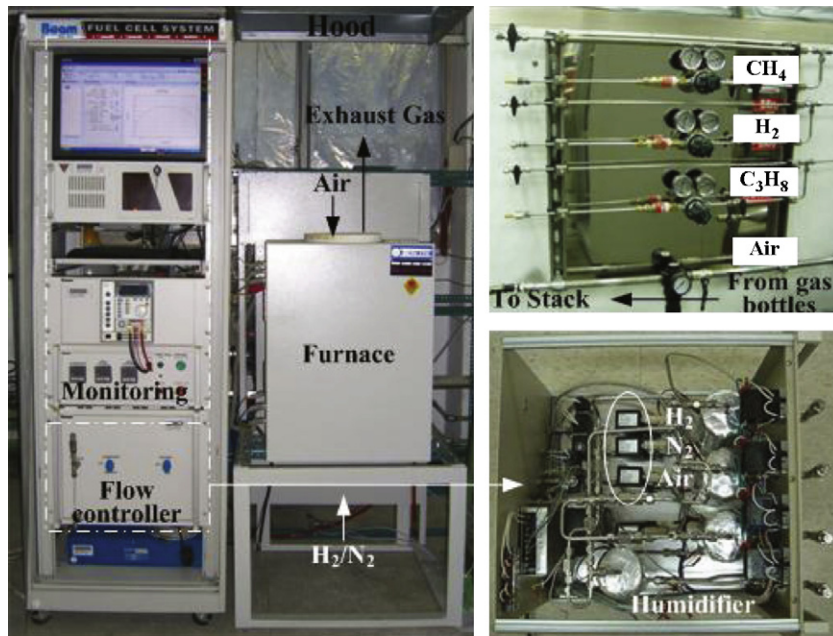
Fig. 2. A SOFC testing platform including a furnace in which the single-cell stack is tested, various gas supply valves and lines, the exhaust gas hood, and power measuring devices.
